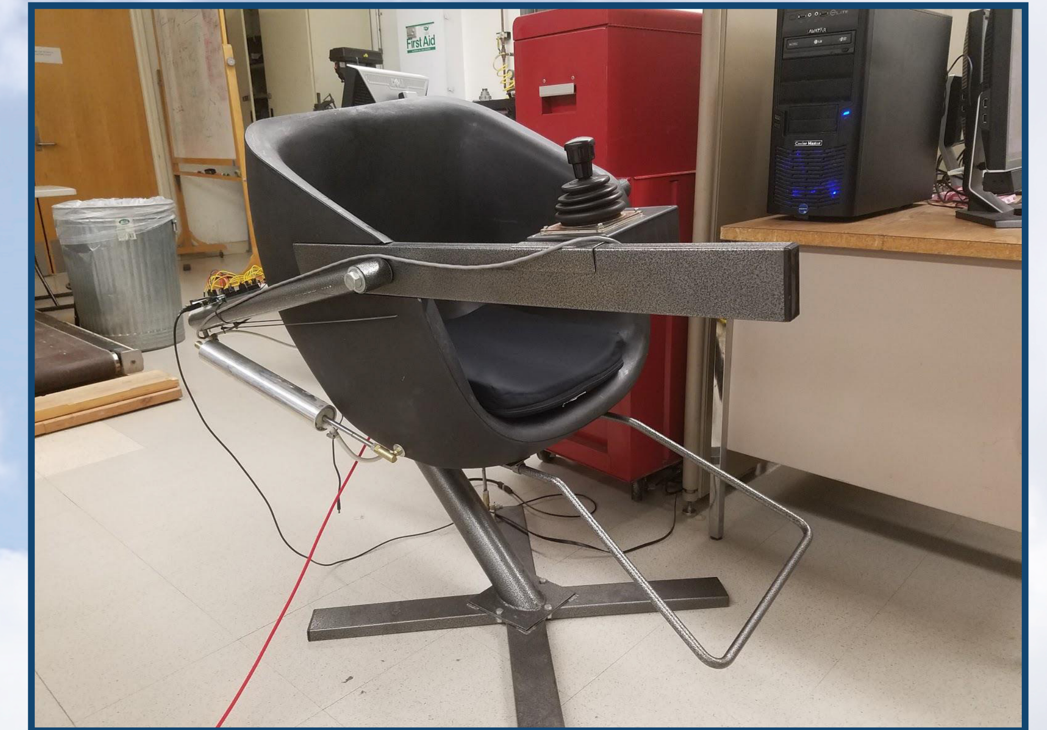
Our current chair uses a computer monitor and does not have any rudder pedals.
