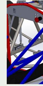
Batteries team began manufacturing the battery box this quarter. Using the tacked box they have checked the fitting of batteries, relays, and fuses. The box will hold 21 batteries in total.
