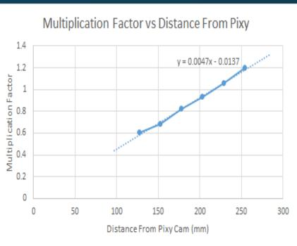
Interpretation: As the distance of the object from Pixy increases, the multiplication factor to obtain proper unit conversion, from Pixy units to mm, increases. This is due to the decrease in registered Pixy units. The following equation will allow us to predict the multiplication factor as the distance increases in order to have accurate units.
