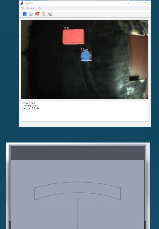
Arm Range Equations  $(X^{2}) + (Y^{2}) = (R^{2})$ 346.85 (mm) < R < 431.55 (mm) 346.85 (mm) < X < 431.55 mm -183.36 (mm) < Y < 183.36 (mm) Y limits set by the imaging range of the top pixy cam X limit determined by the mobility of the arm
